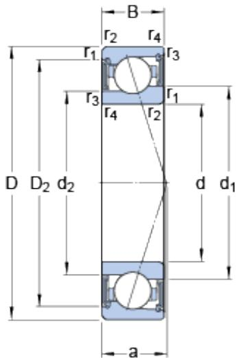
S71911 ACE/HCP4A Bearing 2D drawings and 3D CAD models
